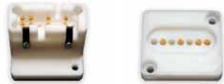
JIG for white goods testing top bottom
