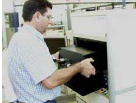
Fixture replacement operation requires less than 2 minutes
