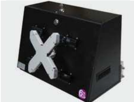
Fixture 7200.7000 configured to test 4 assembled devices with push-buttons and display, simultaneously
