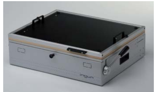
Vacuum Fixture VIN 2040/F/H with Interchangeable Kit ATS VIN 2040
